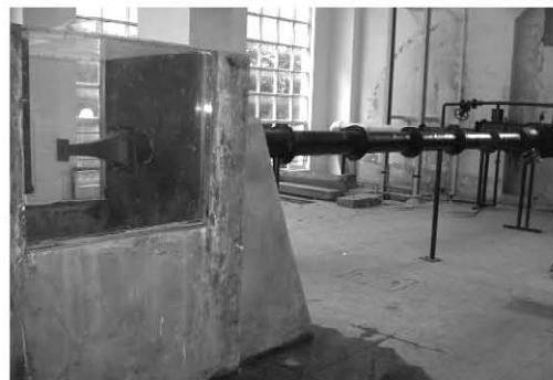
Fig.4 Delivery pipes and test section
